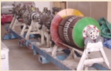
In-Line Inspection tool resting on support tray a few hours before being launched into a pipeline.
